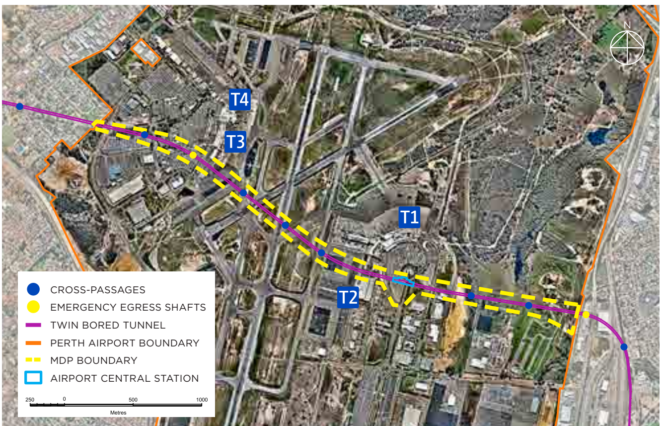
Figure 4.10 Cross-passage locations Source: PTA
